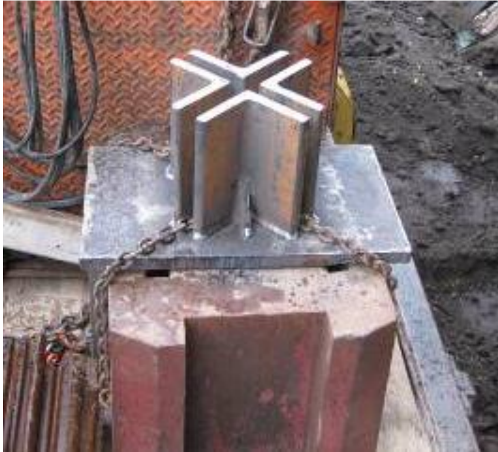
Figure 5-17. Custom sheet pile driving cap fabricated by BHC
