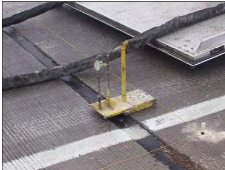
Figure 258. Dial gauge to measure change in approach slab elevation
