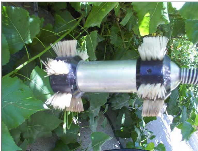
Figure 244. Snake camera used to inspect subdrains
