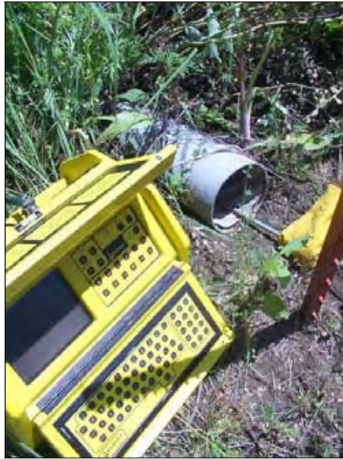
Figure 245. Control of snake camera
