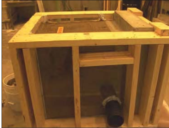
Figure 365. Granular backfill placed behind the abutment
