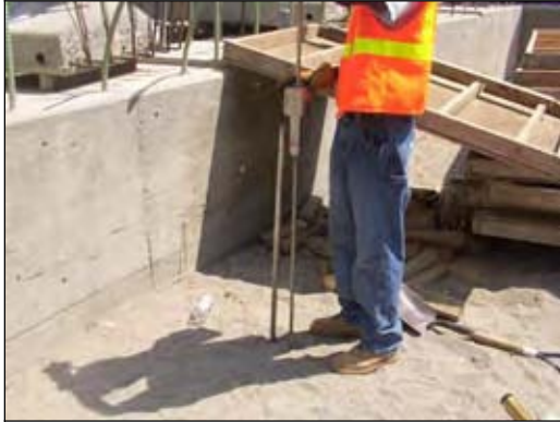
Figure 202. DCP and Nuclear gauge tests (South end of NBL)
