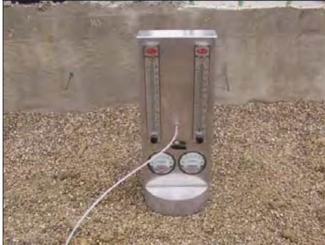
Figure 188. Air Permeability Test performed at porous backfill
