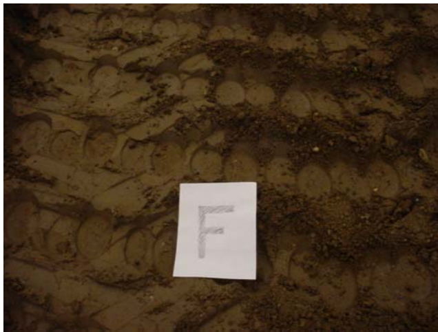
Figure 38. Surface condition after compaction for Test Strip F
