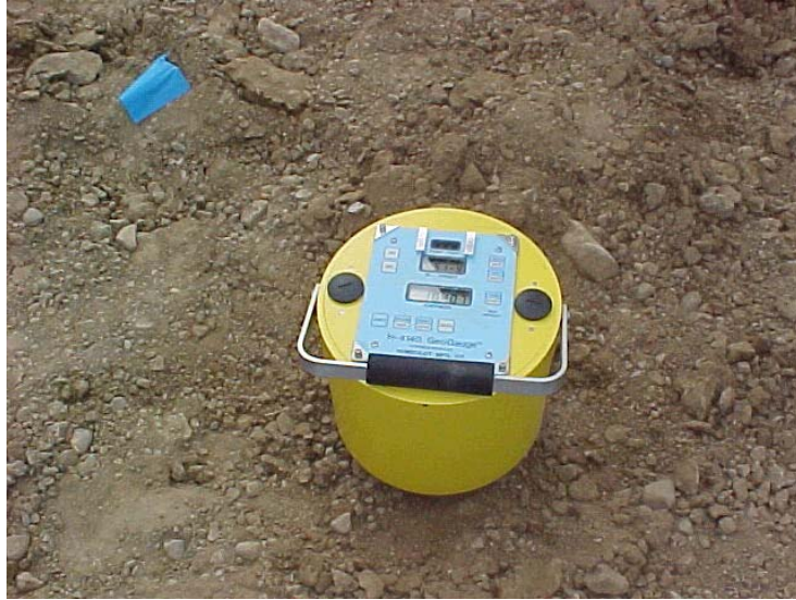
Figure 14. GeoGauge stiffness measurements
