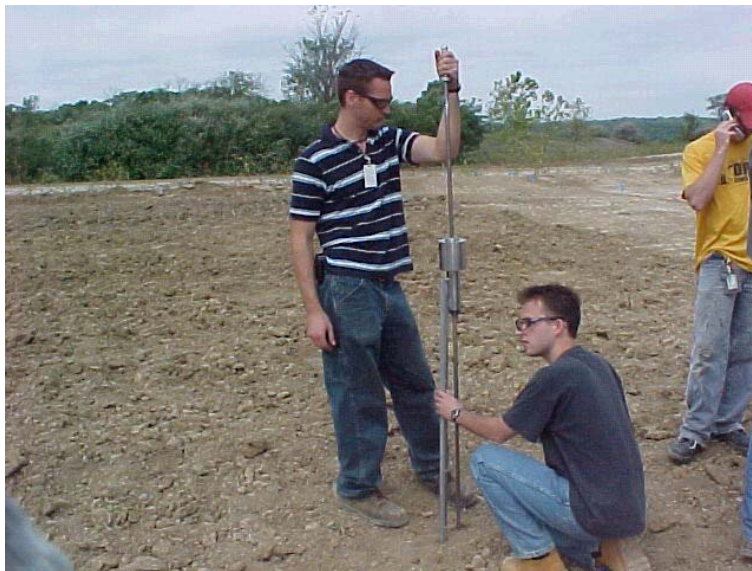
Figure 15. DCP strength profile measurements
