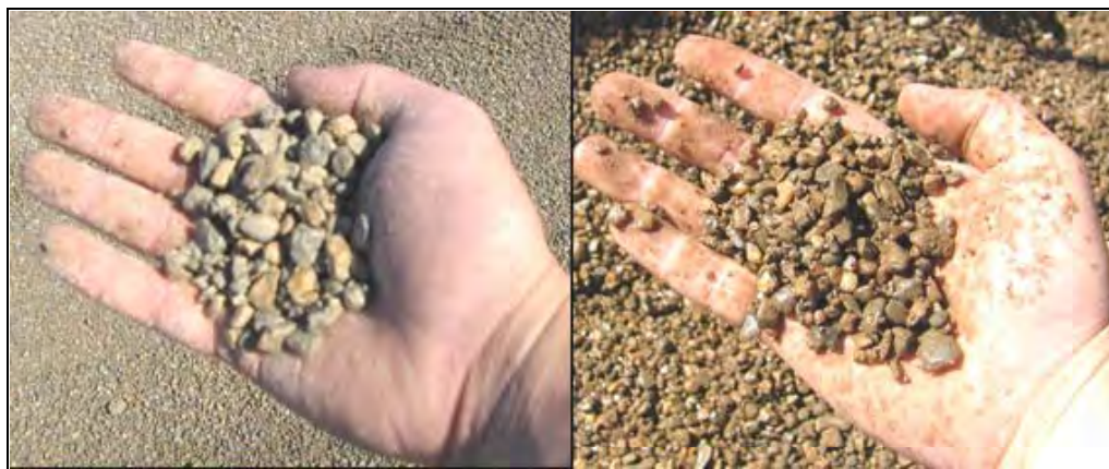
Figure 31. Dusty washed limestone and dirty pea rock chips
