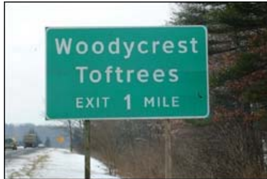
Figure E-5. Sign near Penn State that uses the Clearview road sign typeface
