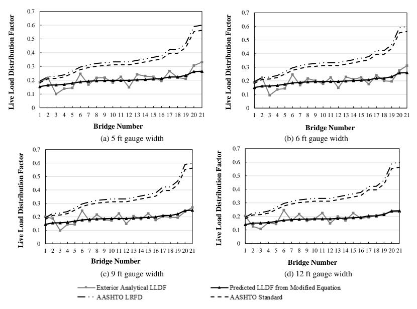
Figure 36(a-d). Exterior analytical LLDF with variation in gauge width – multiple traffic lane steel-timber bridges
