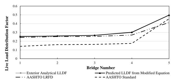
Figure 22. Exterior analytical LLDFs with 121 farm vehicles - one-way traffic lane steelconcrete bridges
