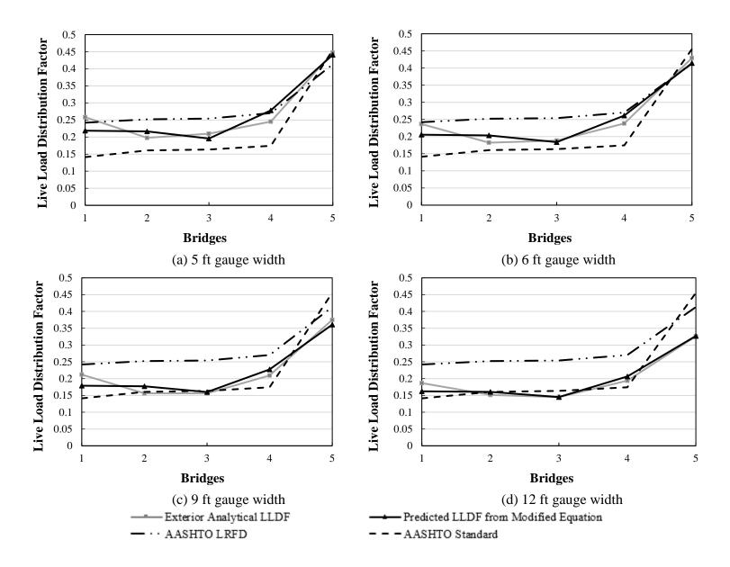
Figure 26(a-d). Exterior analytical LLDFs with variation in gauge width – one-way traffic lane steel-concrete bridges
