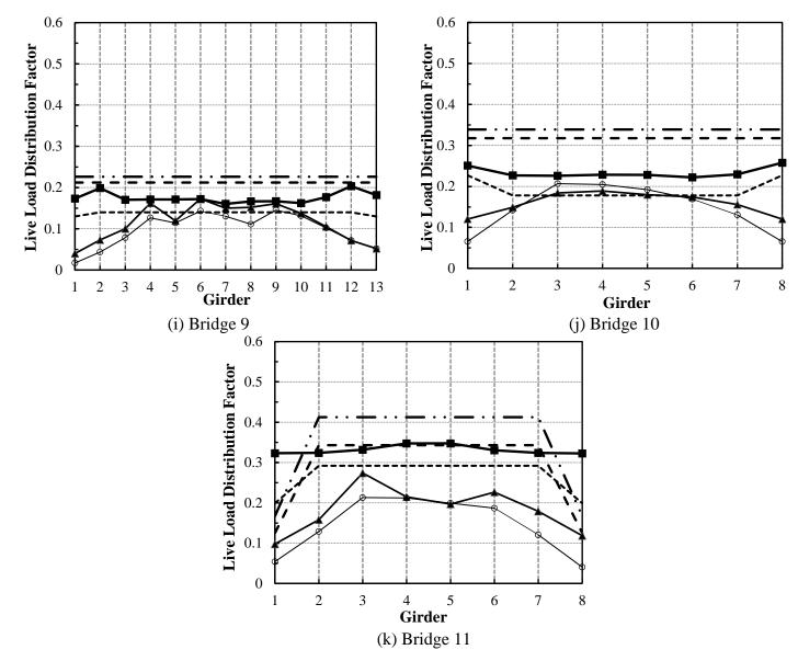
Figure 16(a-k). LLDFs for field-tested steel-timber bridges
