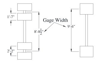
Figure 12. Axle gauge width measurement for two types of axles
