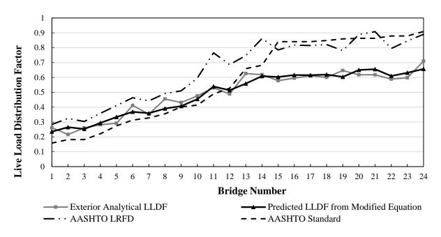
Figure 24. Exterior analytical LLDFs with 121 farm vehicles – multiple traffic lane steelconcrete bridges
