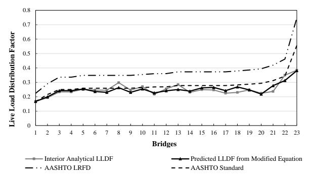
Figure 32. Interior analytical LLDFs with 121 farm vehicles – one-way traffic lane steeltimber bridges
