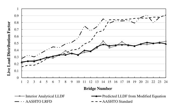
Figure 25. Interior analytical LLDFs with 121 farm vehicles – multiple traffic lane steelconcrete bridges
