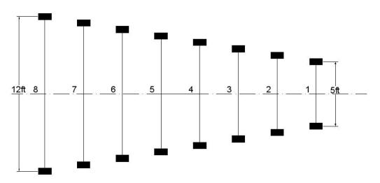
Figure 14. Footprints of eight axles with varying gauge widths of 5 ft to 12 ft
