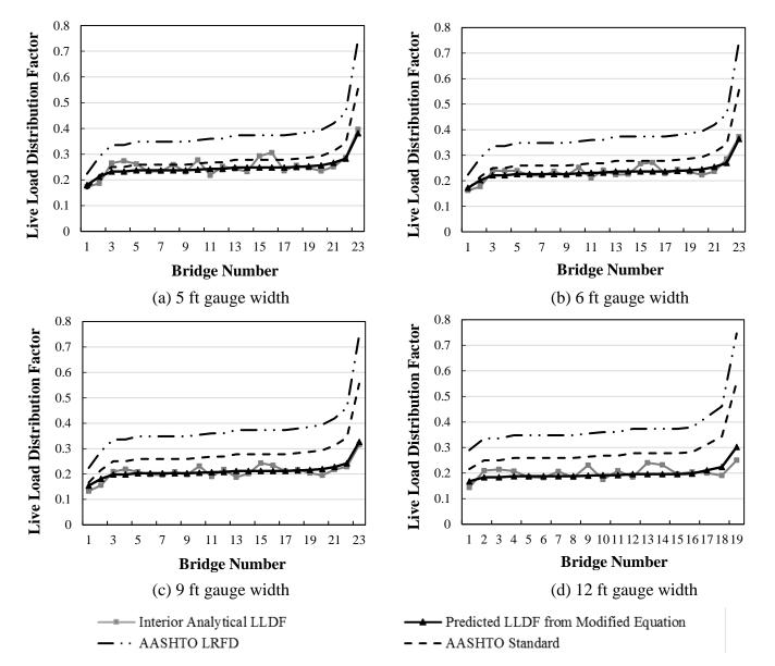
Figure 35(a-d). Interior analytical LLDF with variation in gauge width – one-way traffic lane steel-timber bridges
