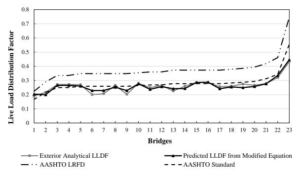
Figure 31. Exterior analytical LLDFs with 121 farm vehicles – one-way traffic lane steeltimber bridges
