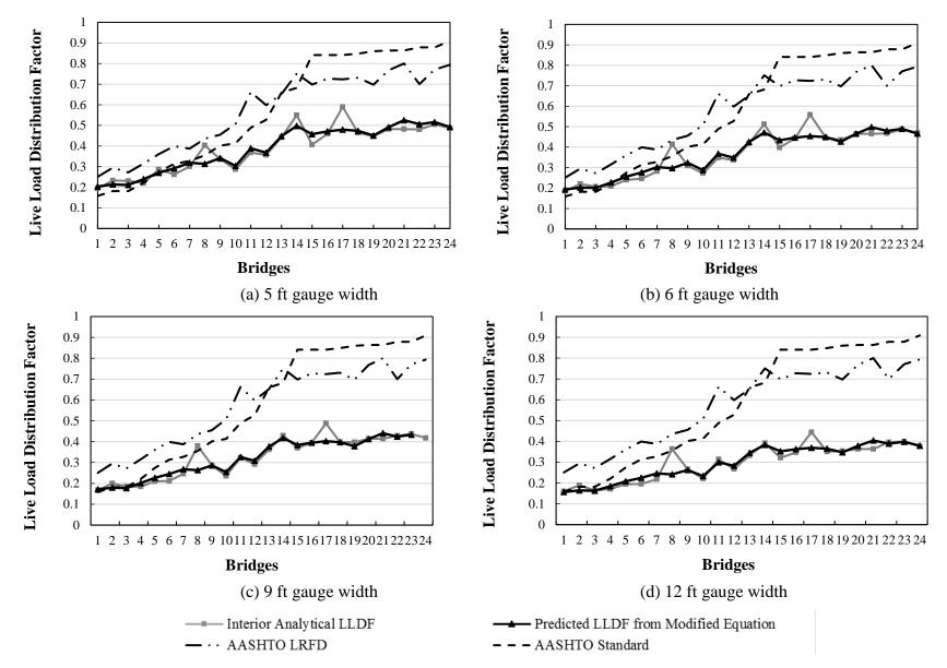
Figure 29(a-d). Interior analytical LLDFs with variation in gauge width – multiple traffic lane steel-concrete bridges
