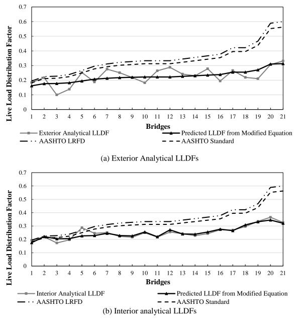
Figure 33(a-b). Exterior and interior analytical LLDFs with 121 farm vehicles – multiple traffic lane steel-timber bridges
