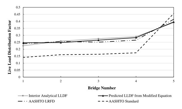
Figure 23. Interior analytical LLDFs with 121 farm vehicles - one traffic lane steel-concrete bridges
