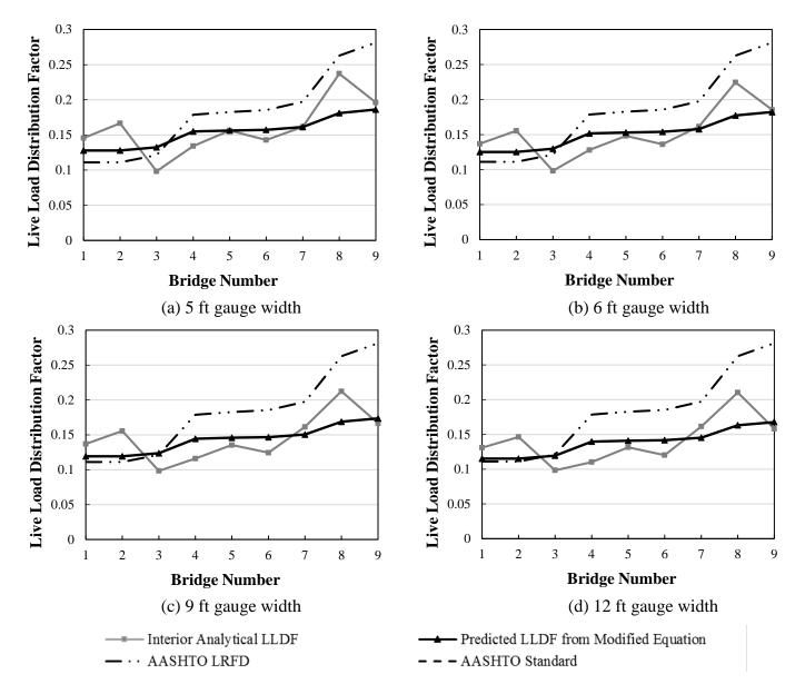
Figure 45(a-d). Interior analytical LLDF with variation in gauge width – multiple traffic lane steel-concrete bridge
