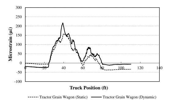
Figure 8. Comparison plot between dynamic and static strain for a representative girder
