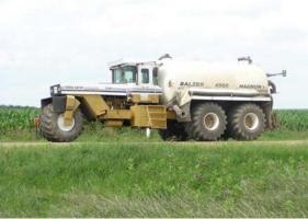
(c1) TerraGator with single-wheel front axle
