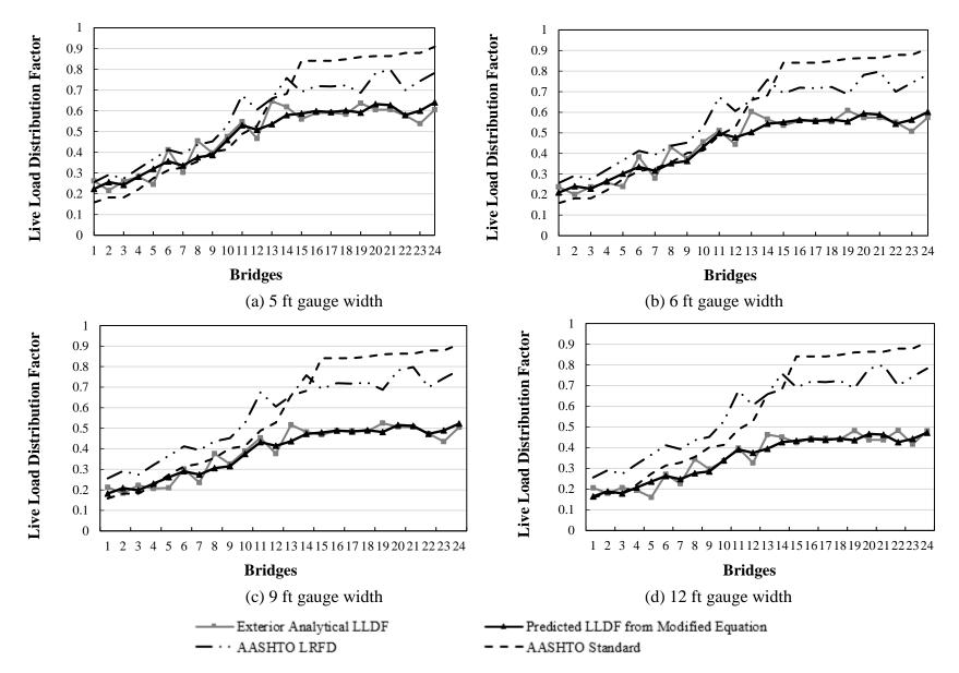
Figure 28(a-d). Exterior analytical LLDFs with variation in gauge width – multiple traffic lane steel-concrete bridge
