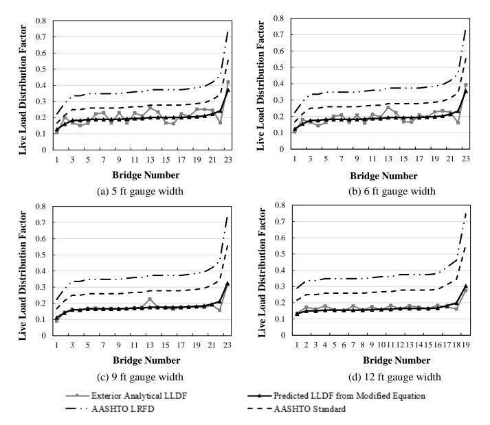
Figure 34(a-d). Exterior analytical LLDFs with variation in gauge width – one-way traffic lane steel-timber bridges
