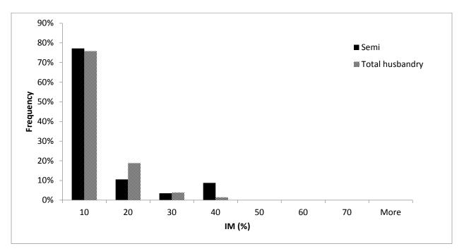
Figure 19. IM frequency for all girders and all vehicles for steel-timber bridges
