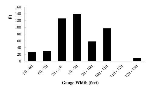
Figure 13. Histogram showing variation of gauge width of farm vehicle inventory
