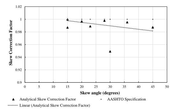
Figure 38 presents the analytical skew correction factors for skewed steel-timber bridges for all 121 farm vehicles.
