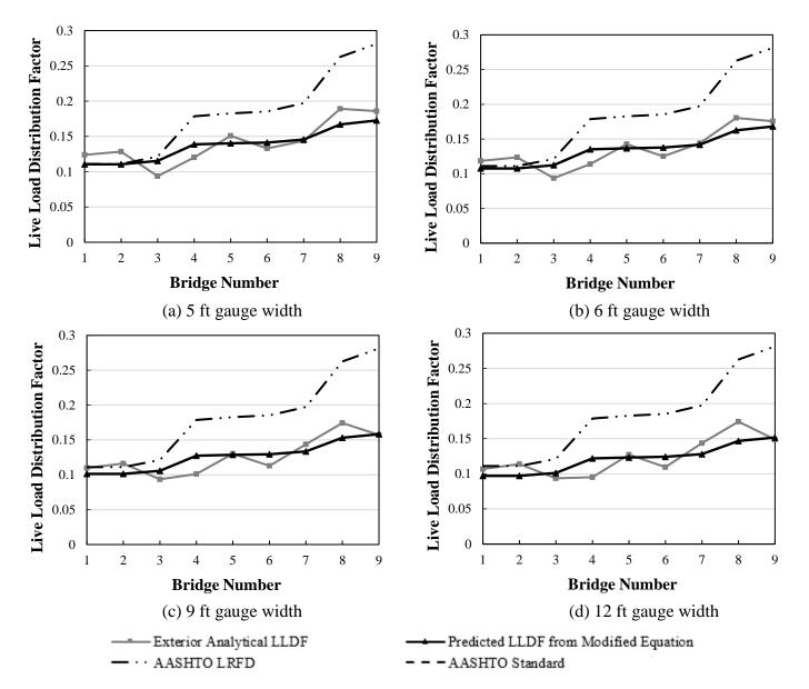
Figure 44(a-d). Exterior analytical LLDF with variation in gauge width – multiple traffic lane timber-timber bridges
