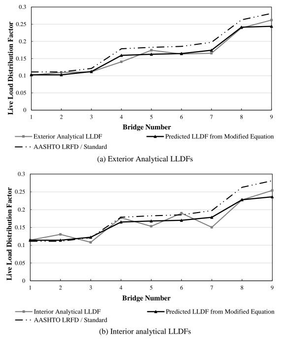
Figure 41(a-b). Exterior and interior analytical LLDFs with 121 farm vehicles – multiple traffic lane timber-timber bridges
