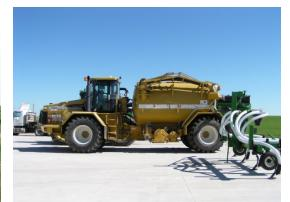
(c2) TerraGator with dual-wheel front axle
