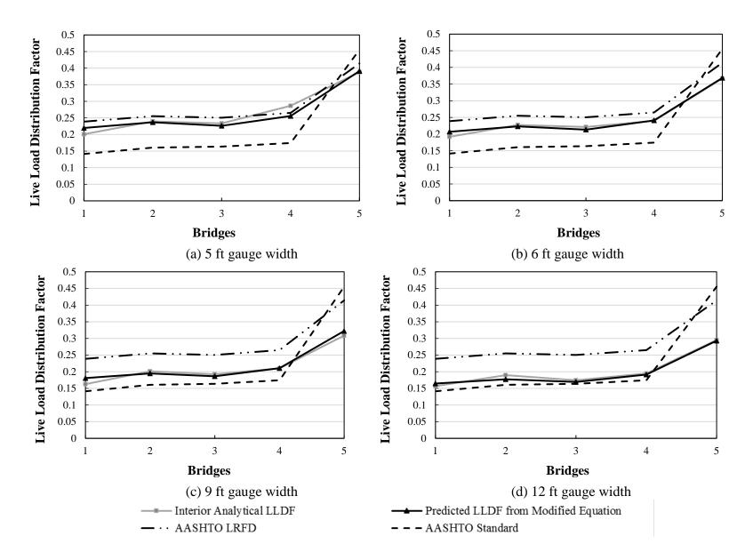
Figure 27(a-d). Interior analytical LLDFs with variation in gauge width – one-way traffic lane steel-concrete bridges
