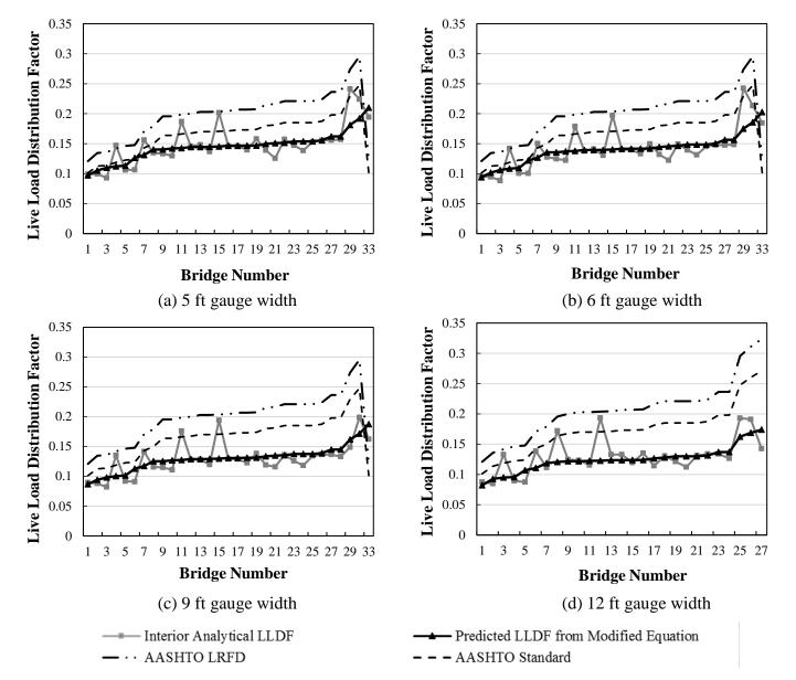
Figure 43(a-d). Interior analytical LLDF with variation in gauge width – one-way traffic lane timber-timber bridges
