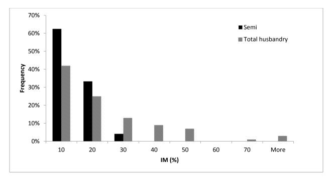
Figure 20. IM frequency for all girders and all vehicles for timber-timber bridges
