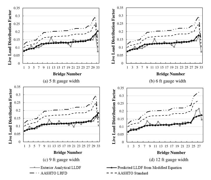
Figure 42(a-d). Exterior analytical LLDF with variation in gauge width – one-way traffic lane timber-timber bridges
