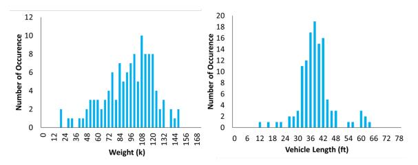
Figure 10. Histograms of vehicle inventory with reference to weight and length
