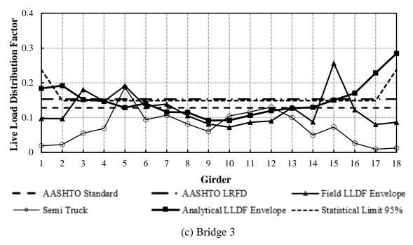
Figure 17(a-c). LLDFs for field-tested timber-timber bridges
