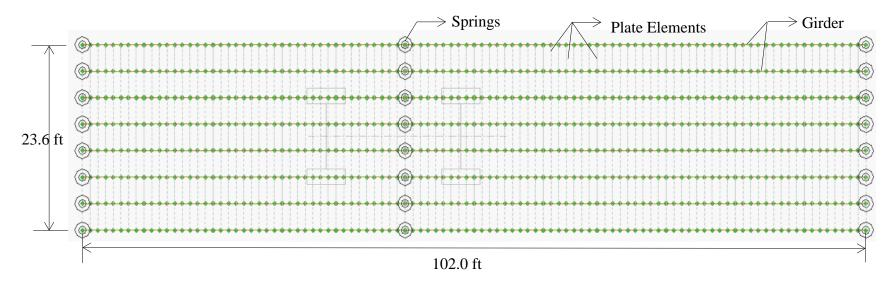
**Figure 9. Finite element bridge model**
