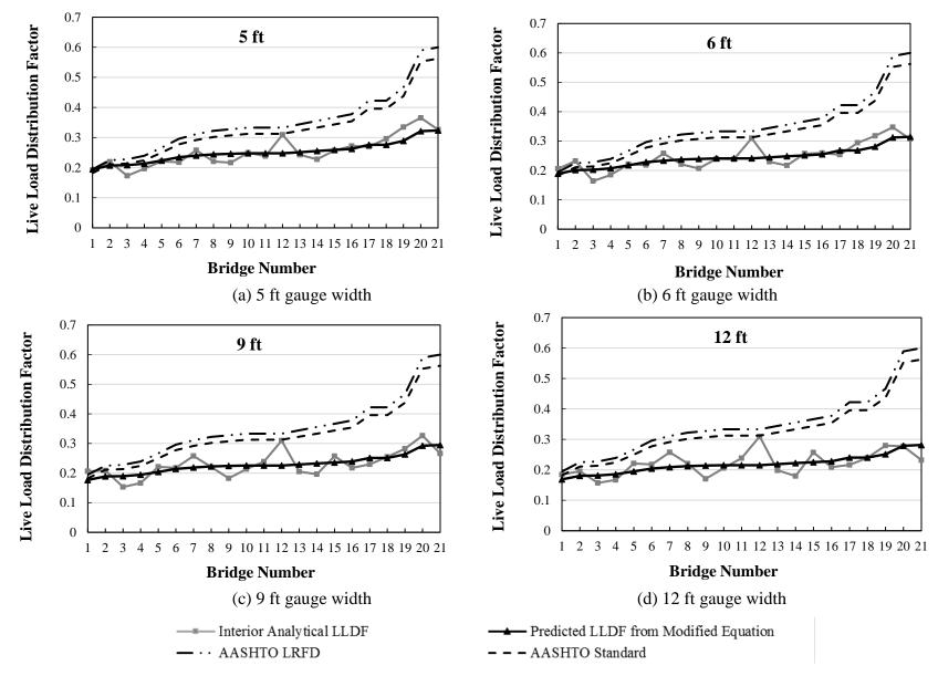
Figure 37(a-d). Interior analytical LLDF with variation in gauge width – multiple traffic lane steel-timber bridges
