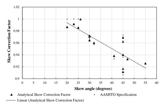
Figure 30. Skew Correction Factors - Steel-Concrete Bridges
