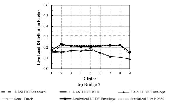
Figure 15(a-e). LLDFs for field-tested steel-concrete bridges
