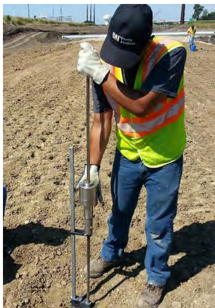
Figure D9. Dynamic cone penetrometer testing (left) and an example plot comparing DCP-CBR profiles in flooded and non-flooded areas
