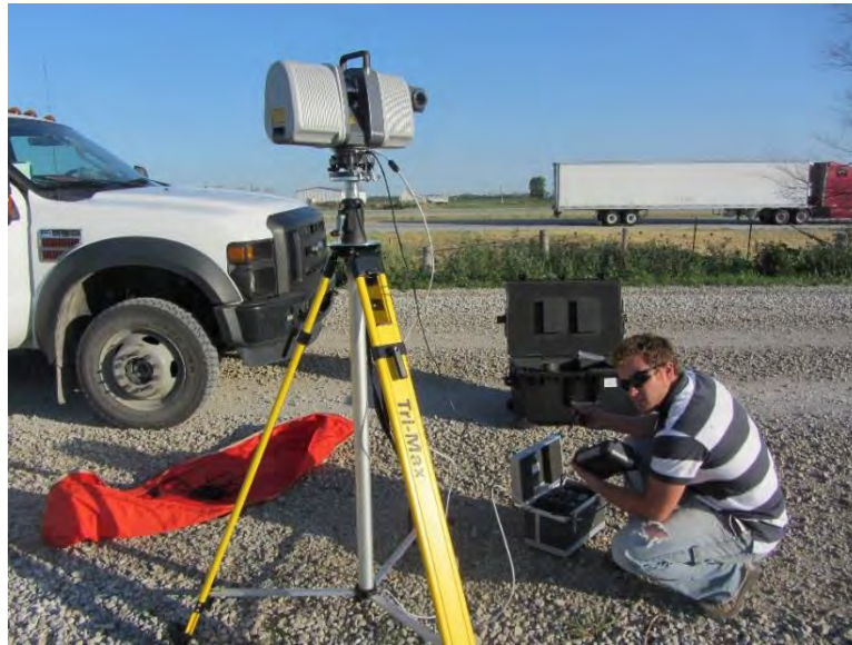
Figure D19. Trimble CX 3D laser scanner
