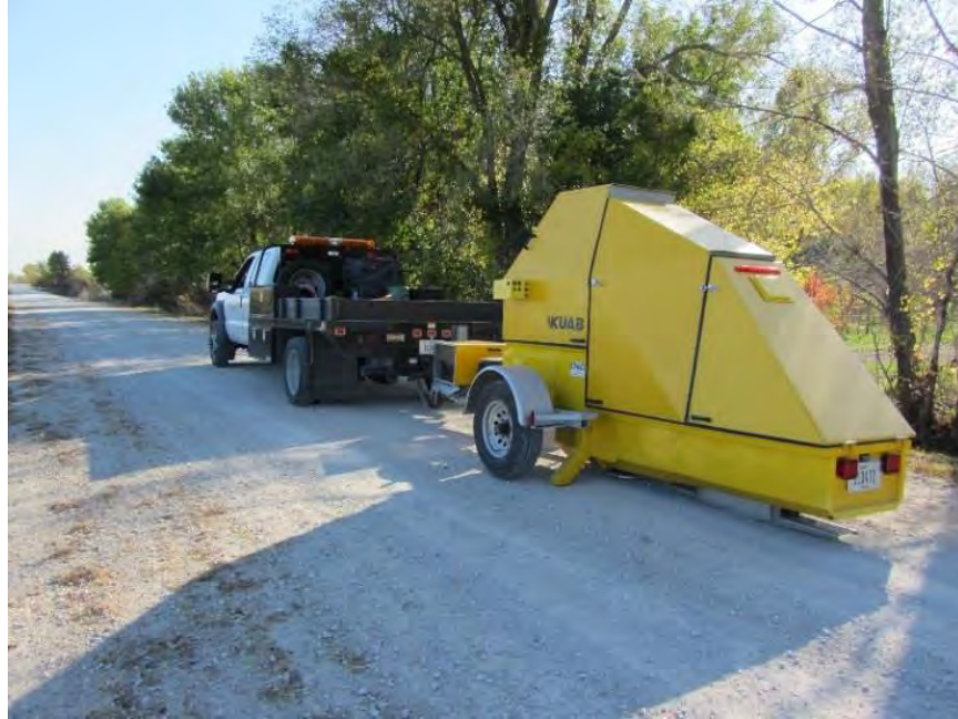
Figure 19. KUAB falling weight deflectometer (FWD)
