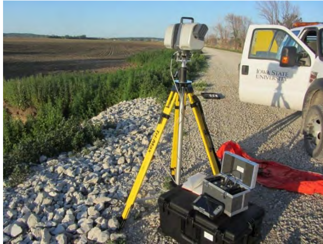
Figure 26. Trimble CX 3D laser scanner
