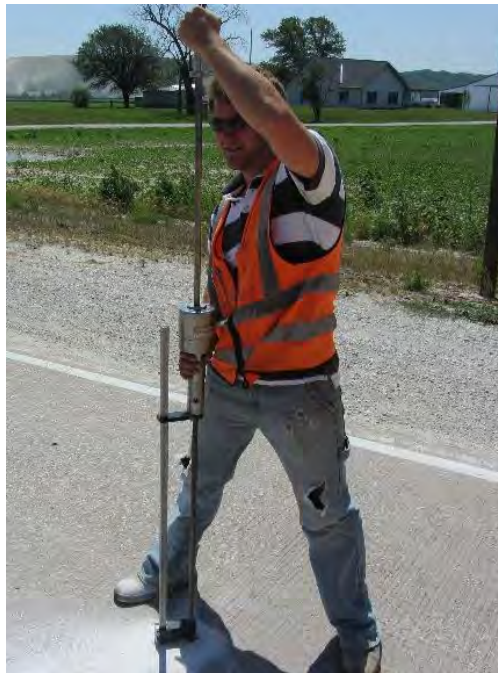
Figure 17. Dynamic cone penetrometer (DCP)
