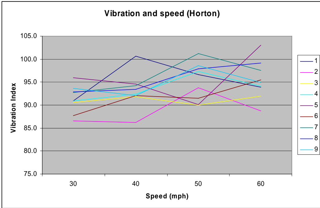
Figure 71. Vibration and speed for various strip types and configurations.
