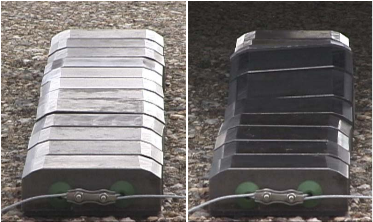
Figure 58. Bounce of 4-in strip during traversal while braking
