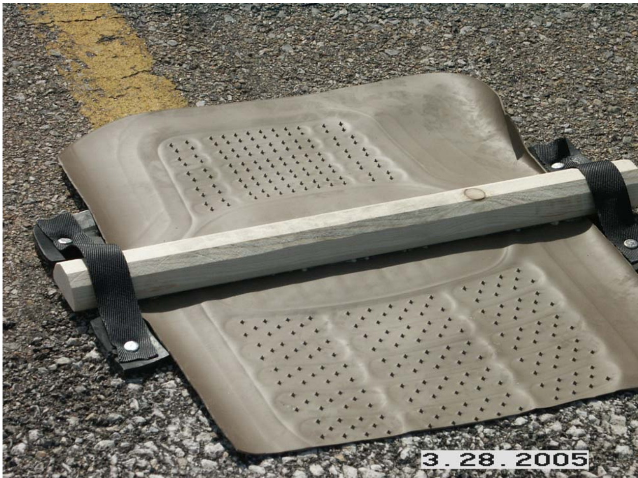
Figure 37. Wooden prototype rumble strip in place for testing.
