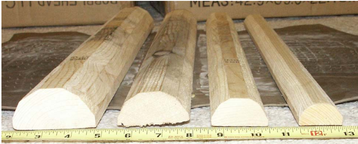
Figure 36. Section view of four sizes of prototype rumble strips, 1.50'' to 0.75'' (L to R).
