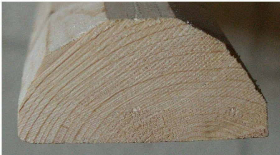
Figure 35. Cross-section of a 1.50"-radius prototype.
