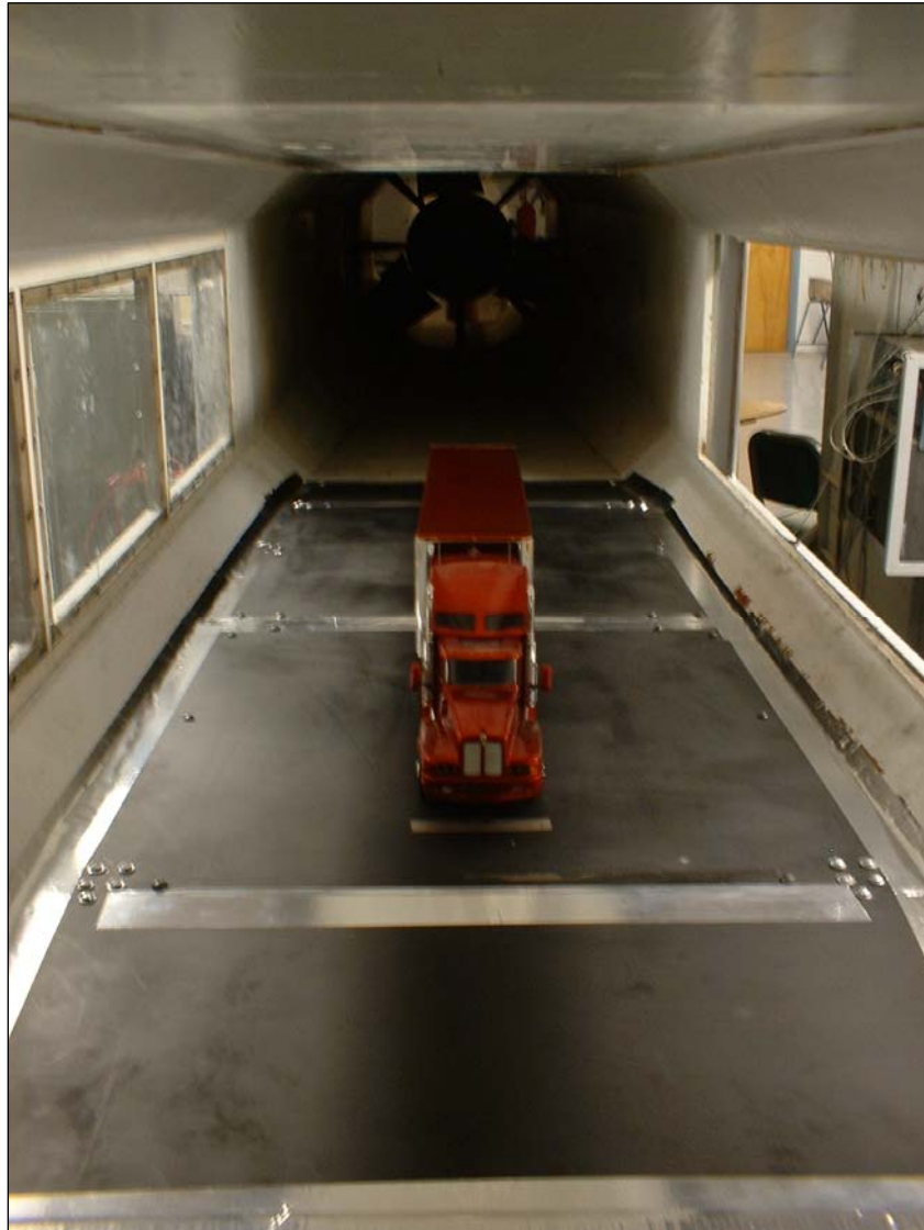
Figure 3. View inside wind tunnel showing model, false floor, ramps, and seal tape.
