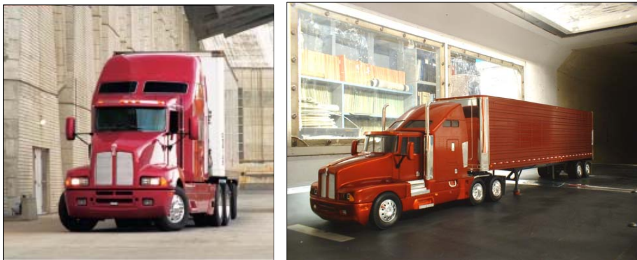
Figure 2. Actual Kenworth T600 (left) and 1/16 scale model (right).
