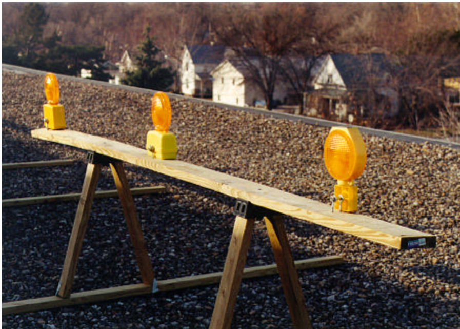
FIGURE 2-2 Array of lights at the testing site. From left to right: battery-powered incandescent, battery-powered LED, and solar-powered LED lights.
