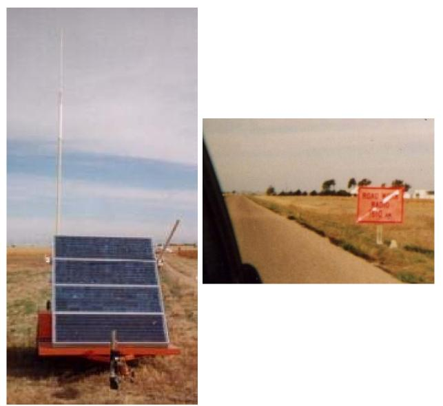
Figure 3. HAR Trailer (front view) showing solar panel (left) and "Road Work / Radio / 1610AM" Sign (right).
