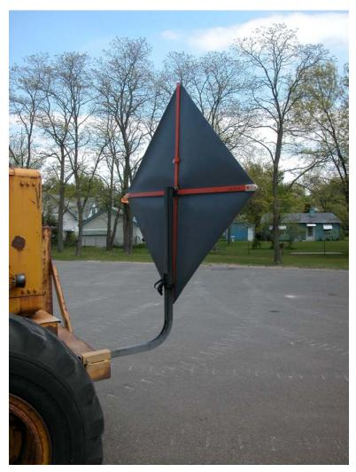
Figure 1. Rollup Sign and Holder with Pin Bracket on Rear of a Grader
