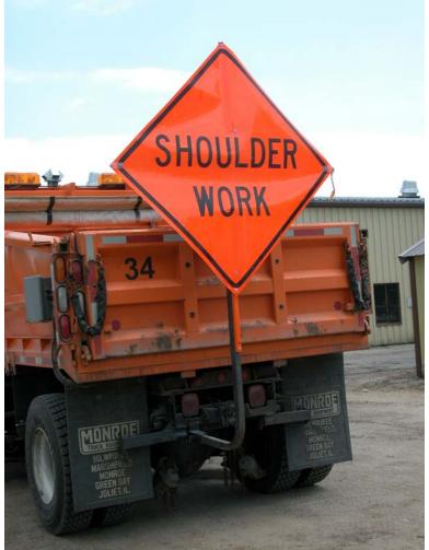
Figure 4. Rollup Sign and Holder on Rear of a Truck
