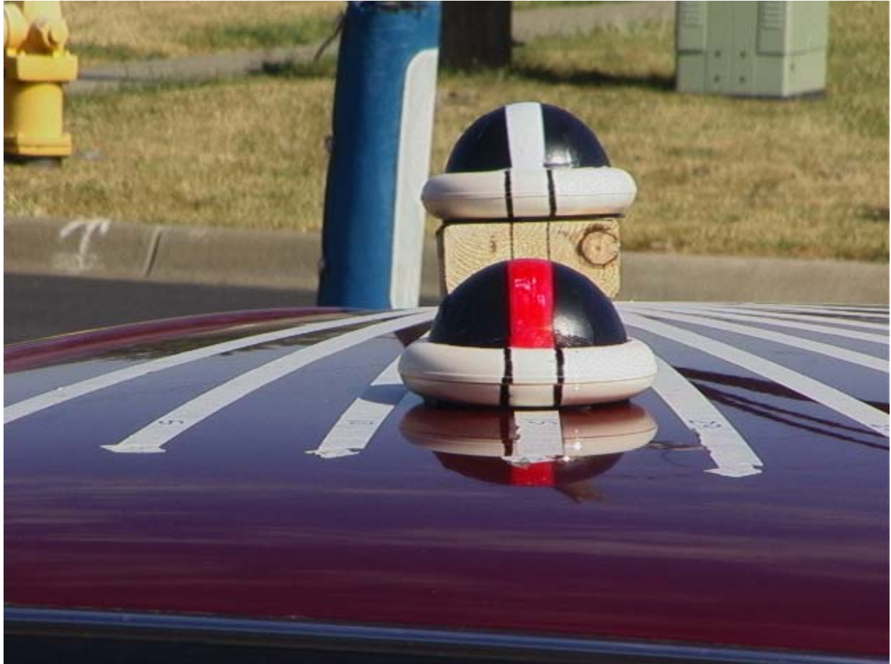
Figure 7. Spotters perspective of markers when aligned. (Shown during daylight for illustration purposes.)
