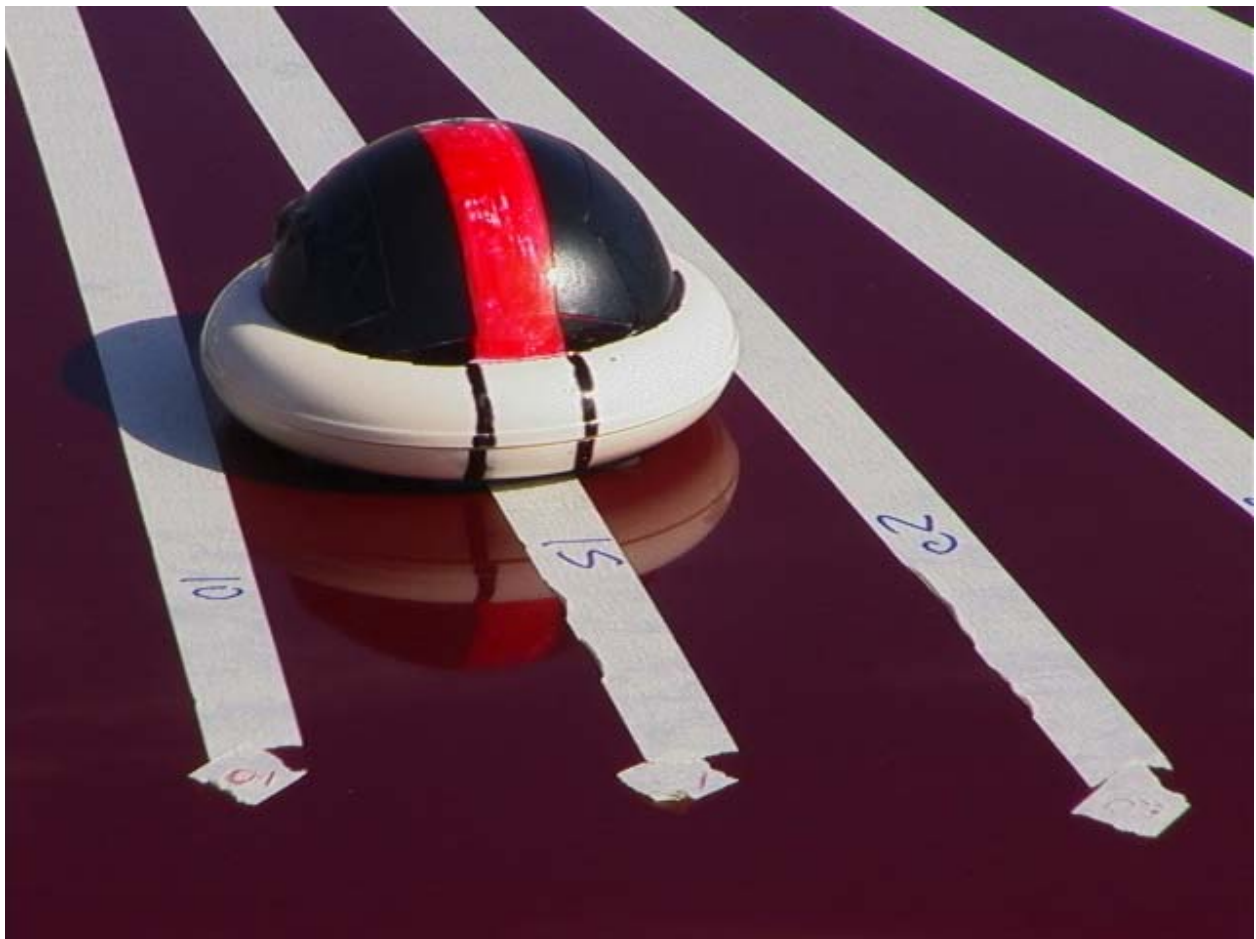
Figure 6. Forward marker set to indicate 15 degrees eccentricity. (Shown during daylight for illustration purposes.)
