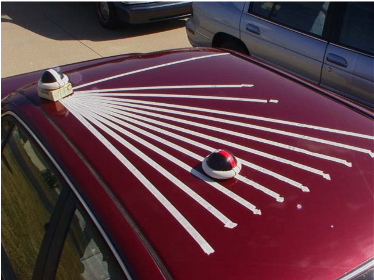
Figure 5. Eccentricities mapped out on the roof of the test vehicle. (Shown during daylight for illustration purposes.)
