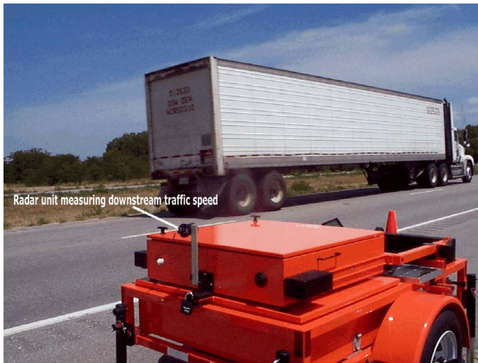
FIGURE 5 Speed Data Collection by Speed Trailers' Radar Unit during "Before" Study
