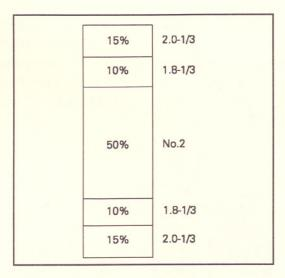
**Figure 1.** Layup configuration for 2400F - 1.8E hardwood glulam timber.
