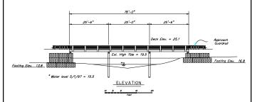
The bridge is designed for AASHTO HS20-44 loading, a bridge length of 76 feet, a width of 16'-3" out-to-out (14'-4" roadway width), and a skew of 0 degrees. The bridge has three spans of 25 feet each, center to center of bearing.
