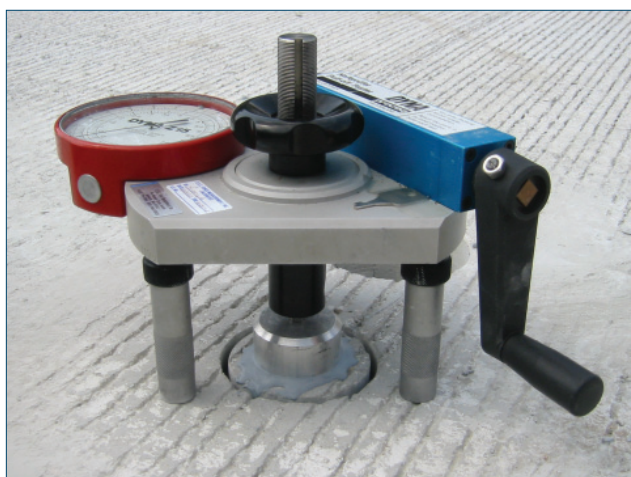
Figure 51. Pull-off test (Photo courtesy of Leif Wathne, P.E., American Concrete Pavement Association)
