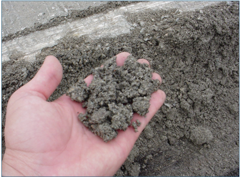
Figure 56. Typical concrete pavement millings from milling operation (Photo courtesy of Dan DeGraaf, P.E., Michigan Concrete Paving Association)
