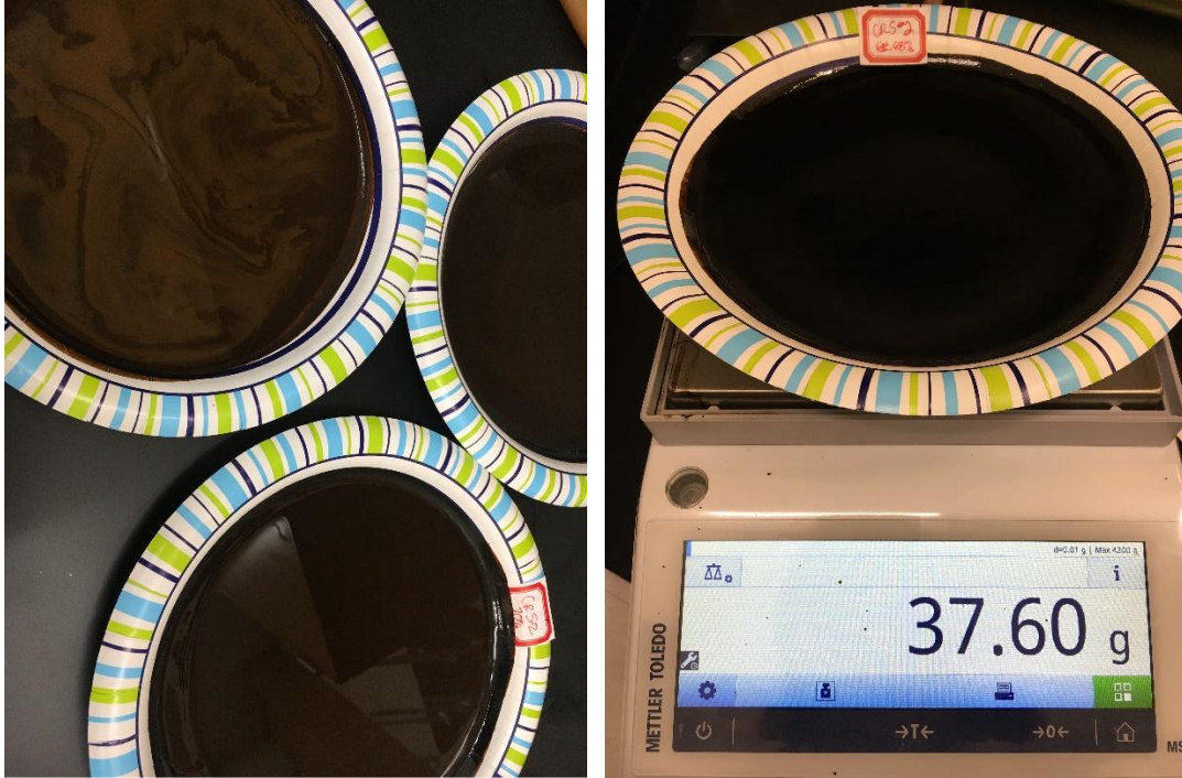
Figure 7. Pouring emulsion samples for residue testing (left) and weighing the residue retained after 24 hours (right)
