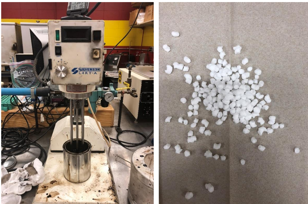
Figure 2. Shear mill for mixing polymers into asphalt binder (left) and SBS polymer (right)
