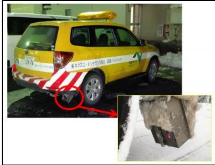
Figure 8. The installation of Yamada-Giken mobile salinity sensor
