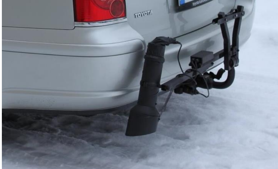
Figure 12. Teconer RCM411 mounted on the rear bumper of passenger vehicle
