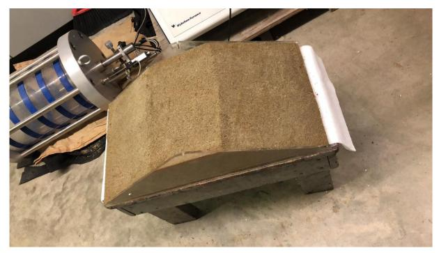
Figure 4. Levee model before testing
