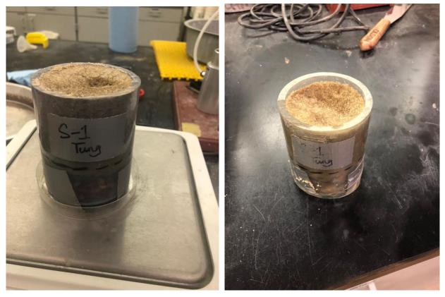
Figure 7. MICP treated specimen after flume test (left) and untreated specimen after flume test (right)
