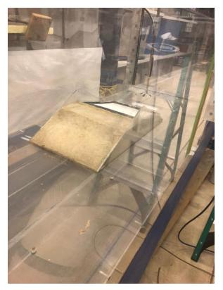
Figure 5. No. 1 levee model flume test set up
