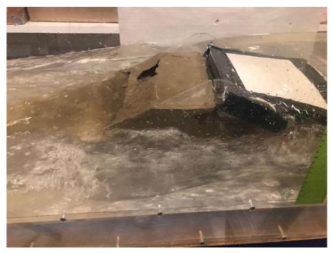
Figure 6. No. 1 levee model during flume test
