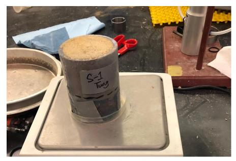
Figure 1. Typical soil column specimen
