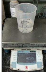
(b) Water removed (429.5 g) during calibration
