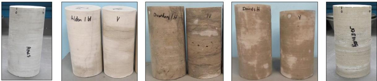
**Figure 3.6. Rock cores for resistivity measurement**
