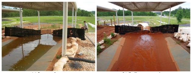
(a) Impoundment(b) Sediment retentionFigure 4.3. Longevity evaluation of pinned silt fence ditch check
