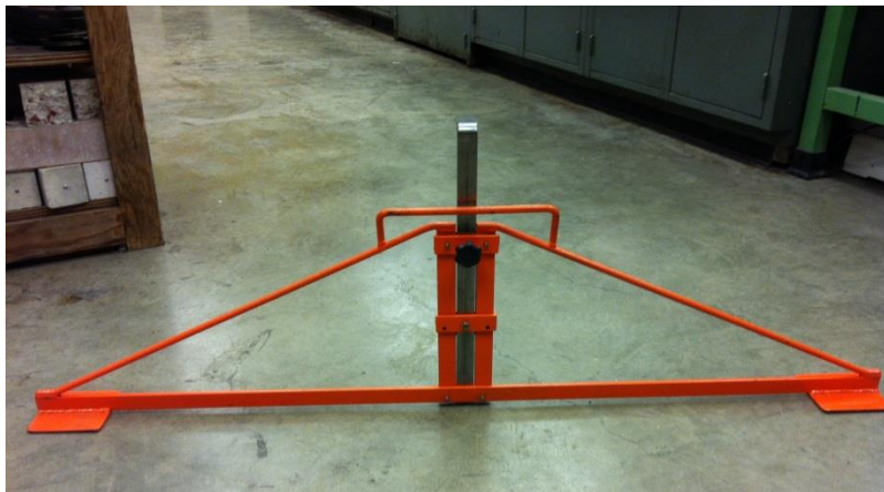
Figure 1. Deflectometer for measuring rutting
