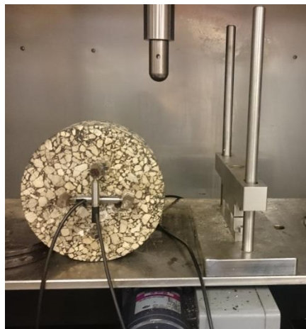
Figure 2. IDT dynamic modulus testing setup
