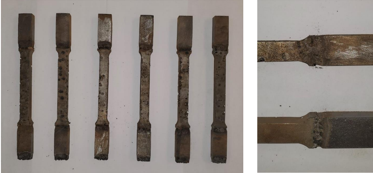
Figure 14. ASTM A1010 corrosion samples
