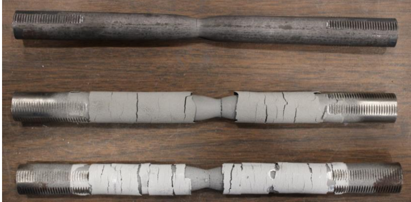
Figure 26. Fractured samples of the A36 coupons with and without cold-sprayed coating after tensile tests
