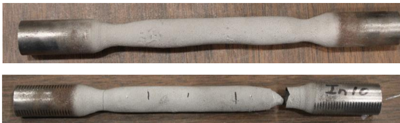
Figure 28. Fractured samples of the corroded A36 coupons with inconel cold-sprayed after tensile tests
