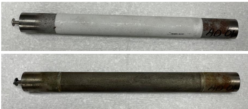
Figure 20. Fourteen-day before and after photos, aluminum
