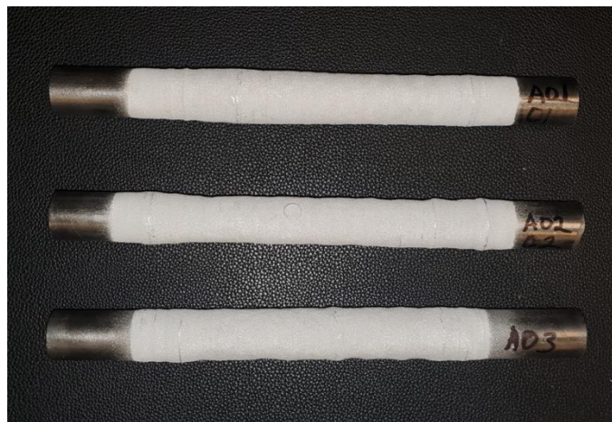
Figure 16. Corroded samples with the mass lost due to corrosion repaired using cold spray coating
