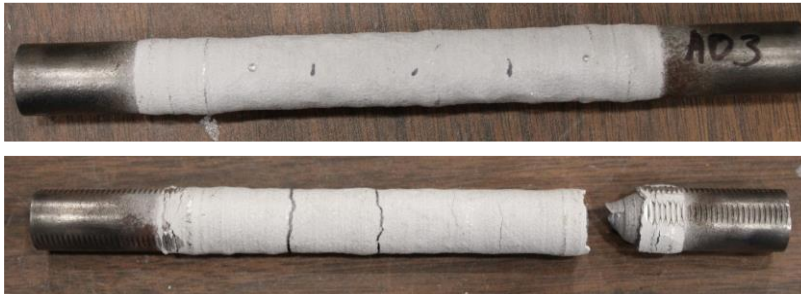
Figure 27. Fractured samples of the corroded A36 coupons with aluminum cold-sprayed after tensile tests
