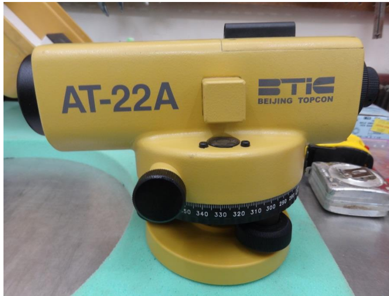
Figure 19. Level for measuring the road profile
