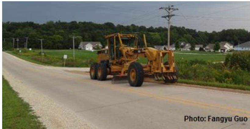
Figure 32. Motor grader used during field tests
