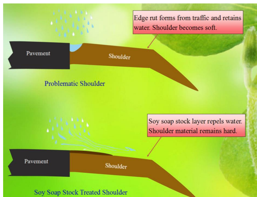
Figure 2. Stabilization of granular shoulders with soybean oil soapstock
