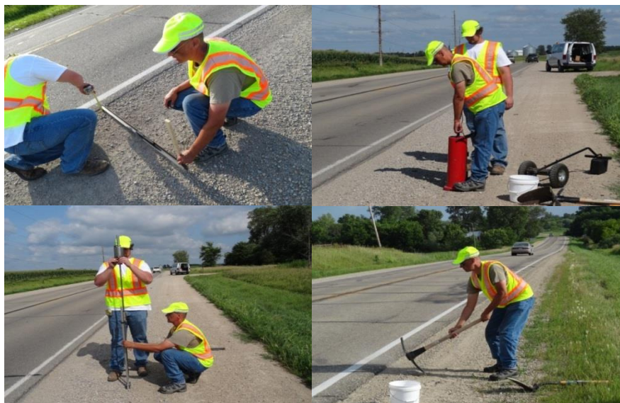
Figure 4. Profile test (top left), Clegg hammer test (top right), DCP test (bottom left), and aggregate samples (bottom right)
