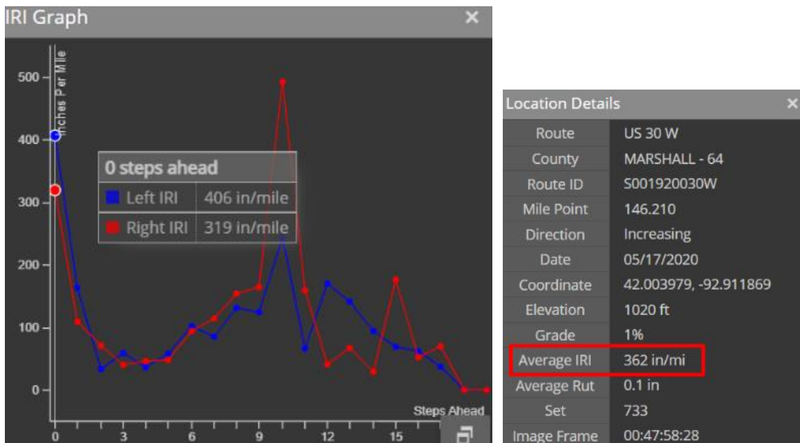
Figure 22. IRI data extraction from PathWeb for bridge 6485.3L030
