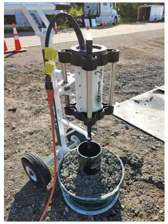
Feedback from some of the states that were provided with VKelly devices was that the system was labor intensive and not user friendly, although in some cases it was felt that the data were valuable. It was reported that a number of operators were using a variety of vibrators and head sizes leading to large variability in the data produced.
