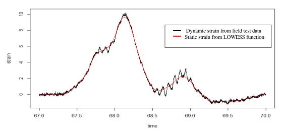
Max Dynamic Strain: 10.2 Max Static Strain: 9.63 DIF: 1.06 Truck weight: Full Lane: Right f=0.05
