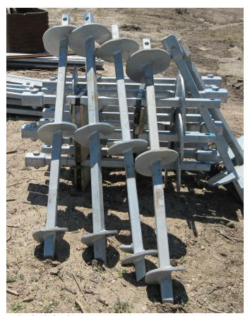
Helical pile lead sections
