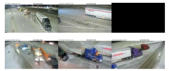
Figure 9. Examples of uncountable cases: missing angle (top), blurry lenses (bottom)
