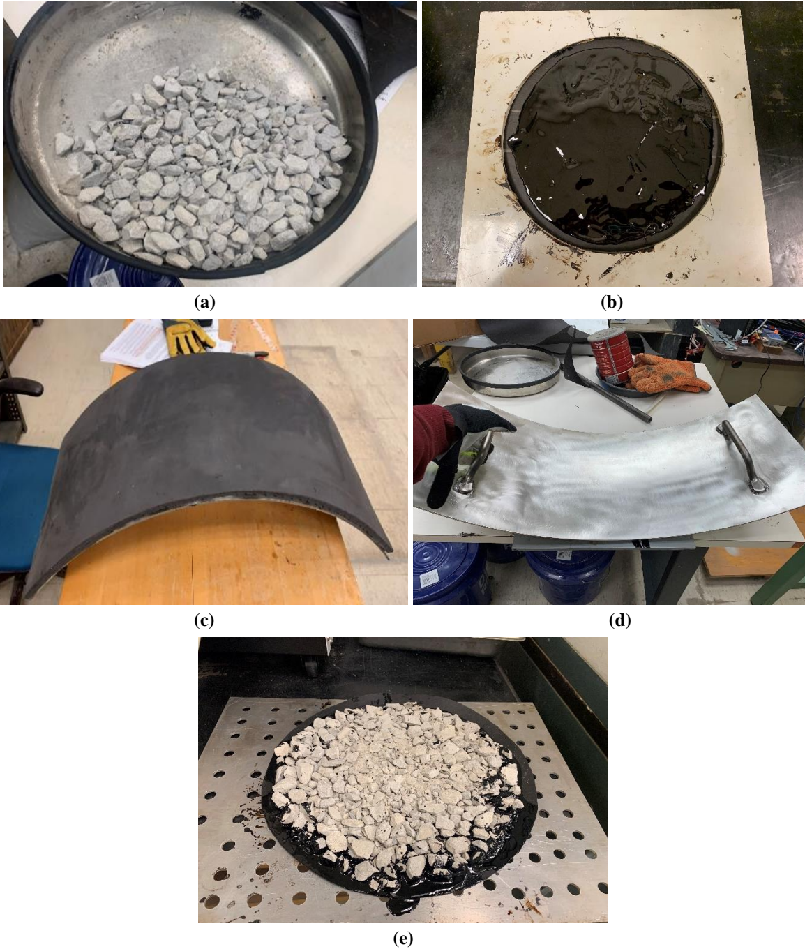
Figure 26. Otta seal specimen preparation: (a) aggregate weighed in pan, (b) binder spread on felt disk, (c) rubber pad on modified steel compactor, (d) top of modified steel compactor, and (e) specimen curing in the oven
