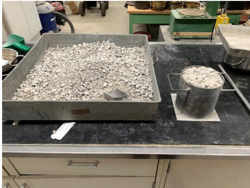
Figure 20. Apparatus used to measure the loose unit weight and voids in loose aggregate
