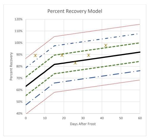
Figure 44. Final model with ±3 standard error bands with 2020 North Dakota Highway 8 data
