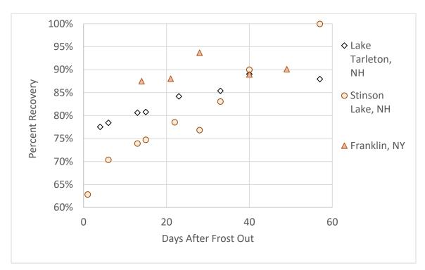
Figure 28. Validation data from three silty sand subgrade sites
