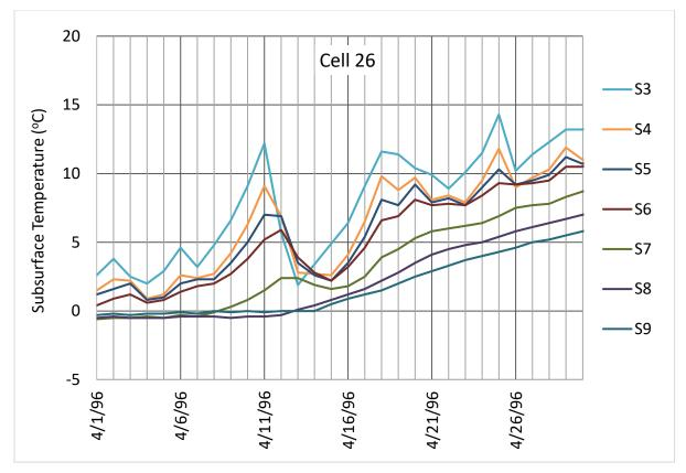
Figure 10. Plot of subsurface temperatures at MnROAD Cell 26 (April 1 through 30, 1996)
