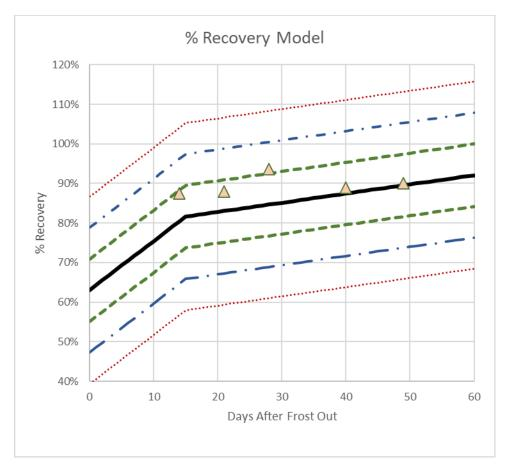
Figure 42. Final model with ±3 standard error bands with 2004 Franklin, New York, data
