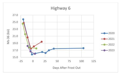
Figure 30. Plot of Ms-36 versus days after frost out at Highway (ND) 6
