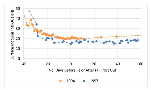
Figure 13. Surface modulus values (Ms-36) from Cell 25 during 1994 and 1997
