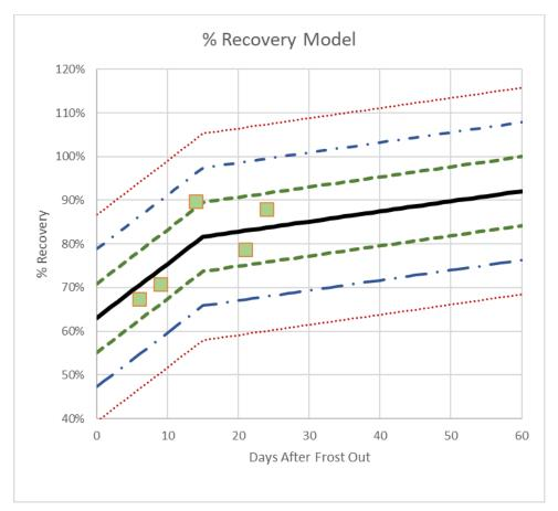
Figure 39. Final model with ±3 standard error bands with 2014 Madison, Maine, data
