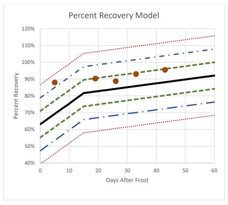
Figure 43. Final model with ±3 standard error bands with 2020 North Dakota Highway 6 data
