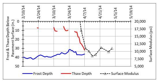
Figure 48. Frost and thaw depths and surface modulus values at Madison, Maine (2014)
