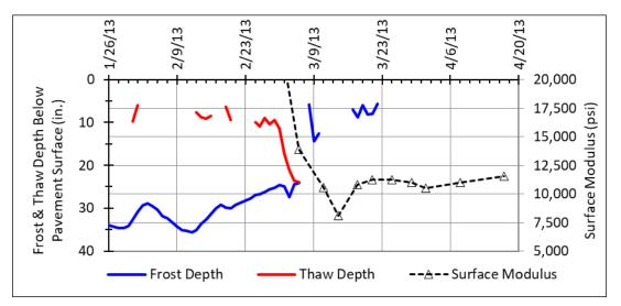
Figure 46. Frost and thaw depths (including secondary freezing) and surface modulus values at Madison, Maine (2013)
