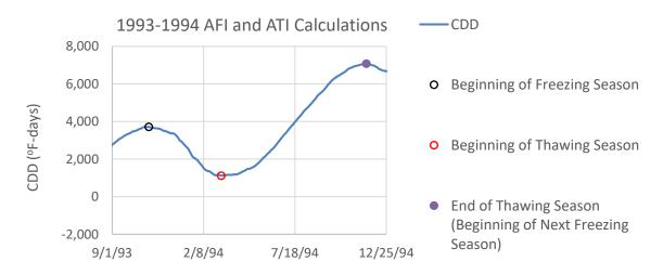
Figure 6. Illustration of AFI and ATI calculations for MnROAD LVR site (1993–1994)
