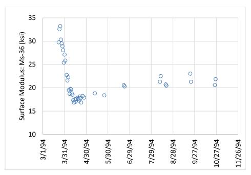
Figure 12. Daily average surface modulus (Ms-36) values from Cell 26 (1994)
