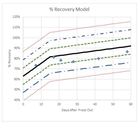
Figure 37. Final model with ±3 standard error bands with Lyme, Jefferson County, New York, data
