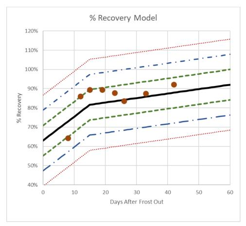
Figure 38. Final model with ±3 standard error bands with 2013 Madison, Maine, data
