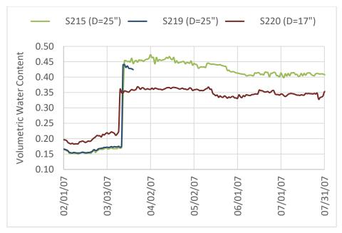
Figure 51. Volumetric moisture content at MnROAD Cell 28 (2007)
