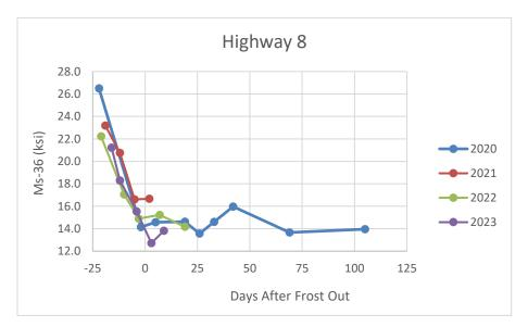
Figure 31. Plot of Ms-36 versus days after frost out at Highway (ND) 8
