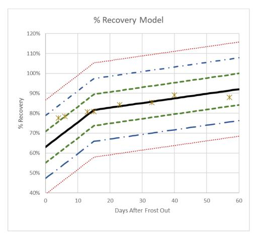
Figure 40. Final model with ±3 standard error bands with Lake Tarleton, New Hampshire, data
