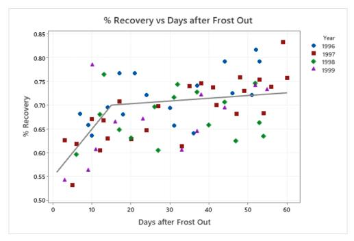
Figure 22. Scatterplot of percent recovery for MnROAD Cell 26 during the years from 1996–1999
