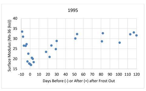
Figure 14. Surface modulus values (Ms-36) from Cell 28 during 1995
