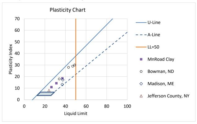
Plasticity Characteristics of Clay Subgrades at Test Sites
