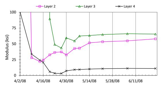
Figure 26. Backcalculated modulus values at Kancamagus Highway site
