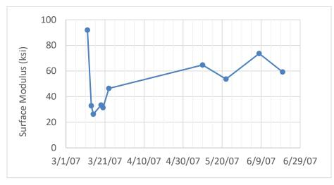
Figure 50. Surface modulus values at MnROAD Cell 28 (2007)
