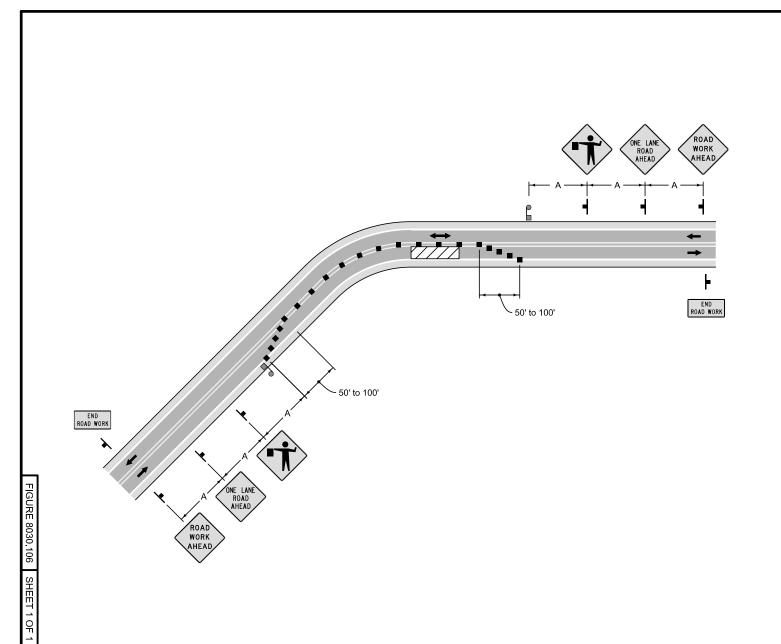
An optional BE PREPARED TO STOP sign may be added between the Flagger sign and the ONE LANE ROAD AHEAD sign.
