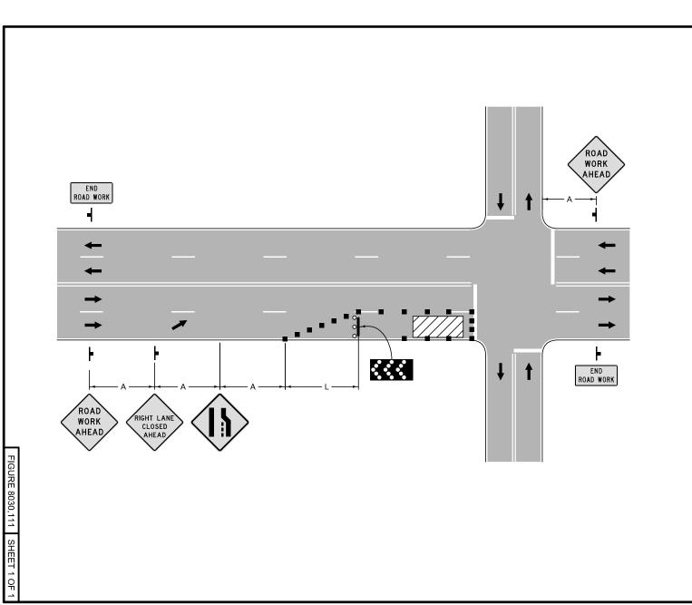
Place arrow board within the closed lane behind the channelizing devices and as close to the beginning of the taper as practical, while keeping it on the paved surface.
