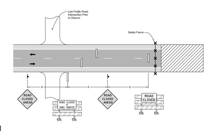
When distance "A" is less than 500 feet, place the barricade with the ROAD CLOSED TO THRU TRAFFIC sign in the middle of the traffic lane approaching the work area. The barricade may be omitted if the distance to the work area is less than 250 feet.
